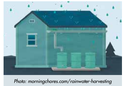
Example of domestic rainwater collection system.
